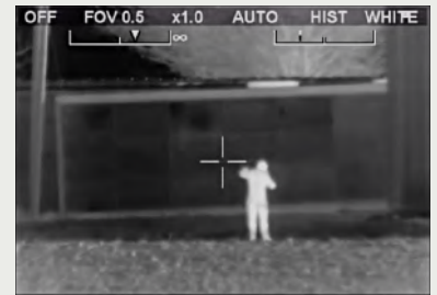
→ Automatic slew-to-cue of identification camera
