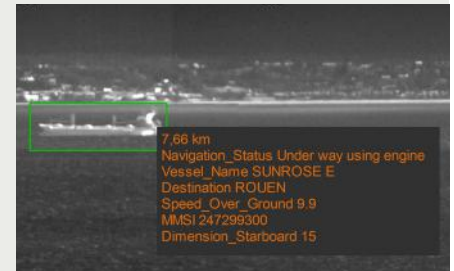
→ Fusion and display of AIS and radar data
